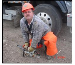
While using a chainsaw, you must follow all proper procedures for its use. Chainsaws must be started properly to avoid injury. Place the saw on the ground and hold firmly while hauling on the starter cord. The saw can also be started in the crotch clamp position. This is done with the rear handle between your thighs, holding the saw with your left hand and pulling the starter cord with your right hand. The "yo-yo" or drop start is dangerous and is not an acceptable method for starting a saw.
