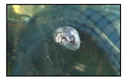
Two pictures, two separate incidents of chain shot on CBPPL operations. In both cases, the chain shot embedded in the lexan glass, which prevented it from entering the cabs. Luckily, no one was hurt in either incident, but that may not be the case in the future. **The best protection is prevention.**
