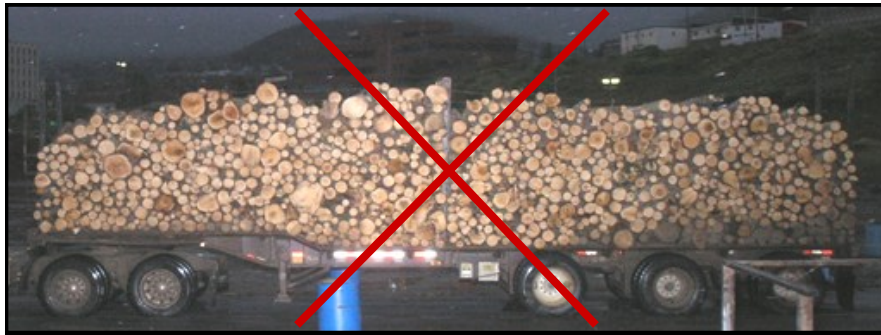
Poor crowning - only 38% contact.
