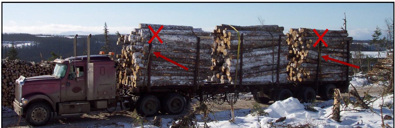
Incorrect placement of tiedowns -they should not cross over stakes.
