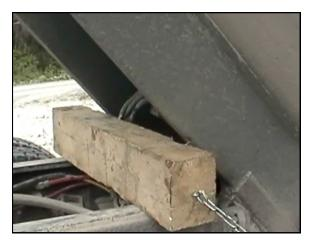
With the dump in the fully-raised position, lay the post across the chassis rails underneath the dump and push it up against the raised dump.
