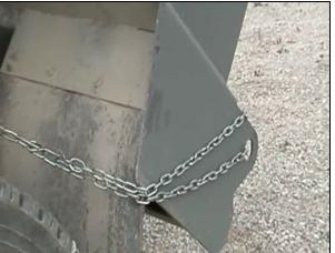
Should the hydraulics fail, the post, held by the chains, will prevent the dump from falling down. Remove the post only when all work is complete.
