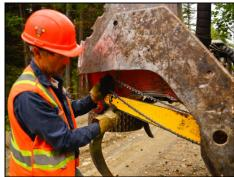
Once the chain and/or bar have been replaced, check the rest of the head for damages or leaks. Check the work area for hazards again, and in Timberjack 1270's, engage the hydraulics before entering the machine. Once safely in the cab, engage the hydraulics (in other than 1270s), start up the machine, and continue cutting.
